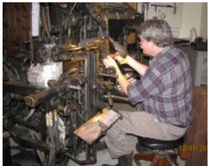
Volunteer Mark Digre tinkers with the linotype machine in the Print Shop. Last fall a traveling machinist repaired a broken part and oiled the machine. It still needs a variety of adjustments before it can cast lead slugs for printing.
